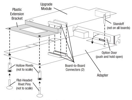
Figure 2-1. Installing an upgrade module on the adapter
